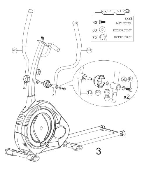
Assemble the left handlebar welding set (52L) & right handlebar welding set (52R) to the main frame (1) using the handlebar post welding set (10), up foot lid (23L), curved washer (75), flat washer (60), angle bolt (40).
