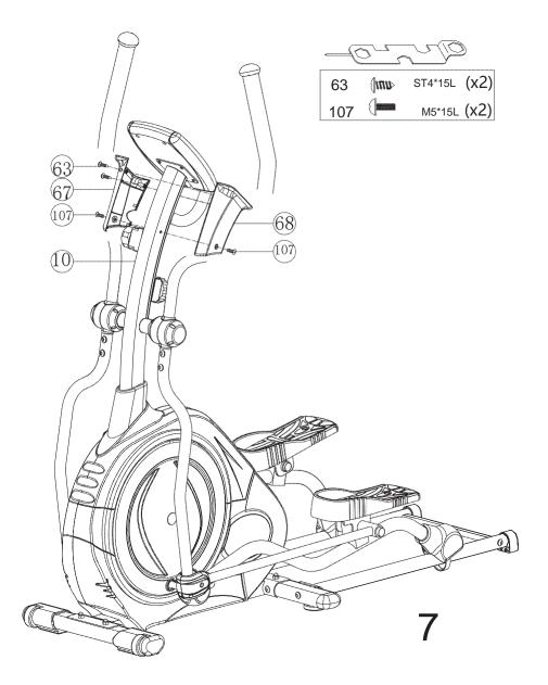
Assemble the computer bracket (67) & computer bracket (68) to the handlebar post welding set (10) using the bolt (107), screw (63).
