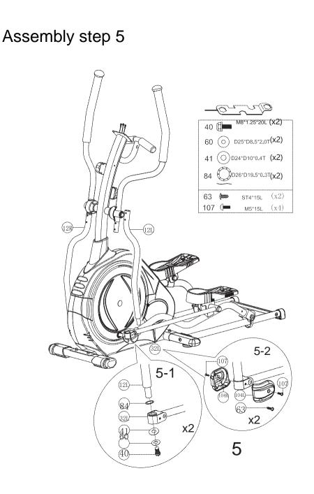
Assemble the right pedal frame welding set (32L) to the main frame (1) using the left sway support tube welding set (12L), curved washer (84), plastic flat washer (41), flat washer (60), six angle bolt (40).
