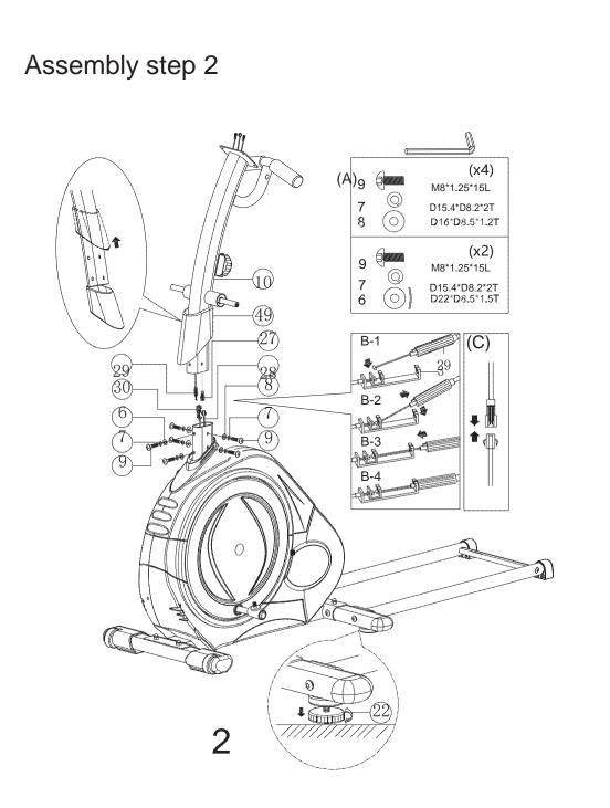
Assemble the (10) to the main frame (1) using the upper protective cover (49), flat washer (8), spring washer (7), inner six angle bolt (9), upper tension cable (27), lower tension cable (28), upper computer cable (29), lower computer (30), curved washer (6).
