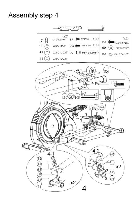
Assemble the left pedal bottom tube welding set (11L) to the main frame
