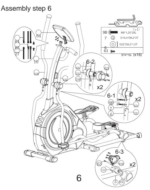
Assemble the left handlebar welding set(52L) to the left sway support tube welding set (12L), inner six angle bolt(9B), spring washer (7), curved washer (6).
