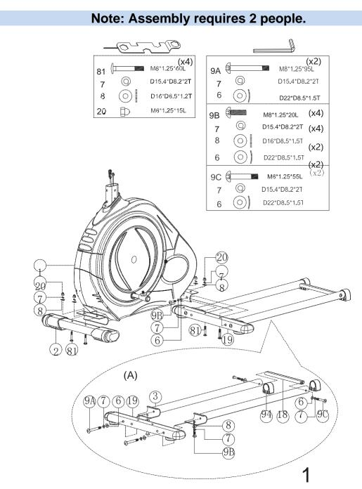
Assemble the front stabilizer welding set (2) to the main frame (1) using the cup nut (20), spring washer (7), flat washer (8), and square bolt (81). Assemble the rear stabilizer welding set (19) to the main frame (1) using the cup nut (20), spring washer (7), flat washer (8), inner six angle bolt (9B), curved washer (6), and square bolt (81).
